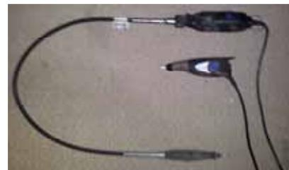
The Dremel uses the extension so you can more easily control the drill bit.
