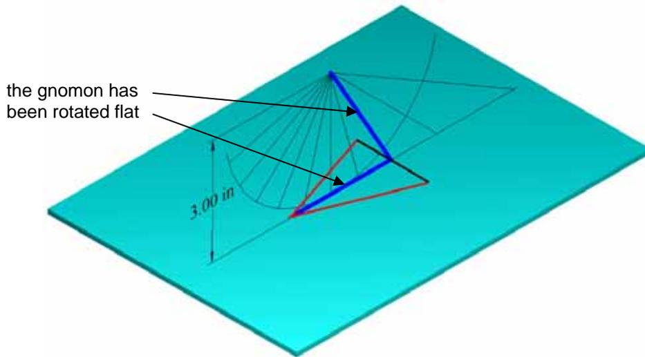
In this case, two hours from noon (30 degrees from the vertical), results in a nodus to dial plate distance that is longer than the one for the preceding noon example.
