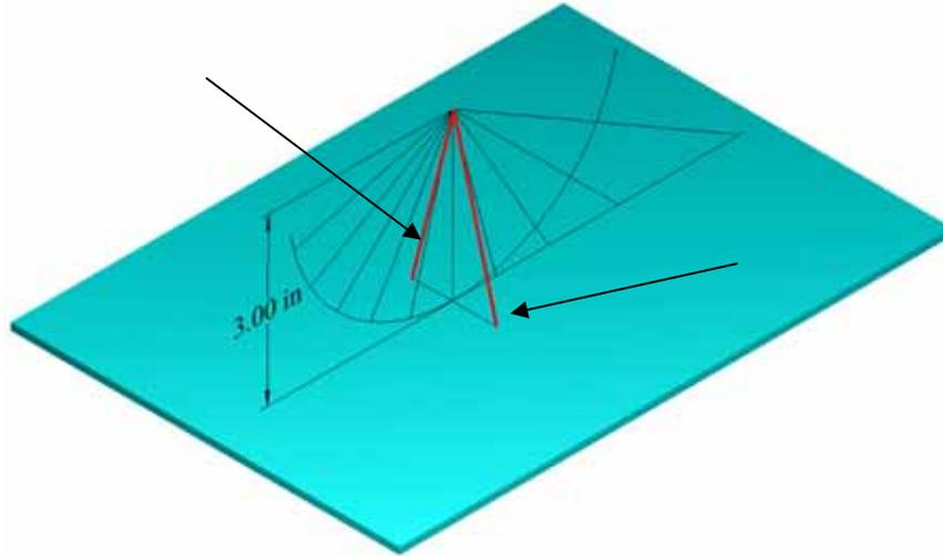
There are two lines which are  $23.44$  degrees from the vertical and show the range of the nodus shadow from the winter to summer solstice, with the equinoxes sharing the straight center line.
