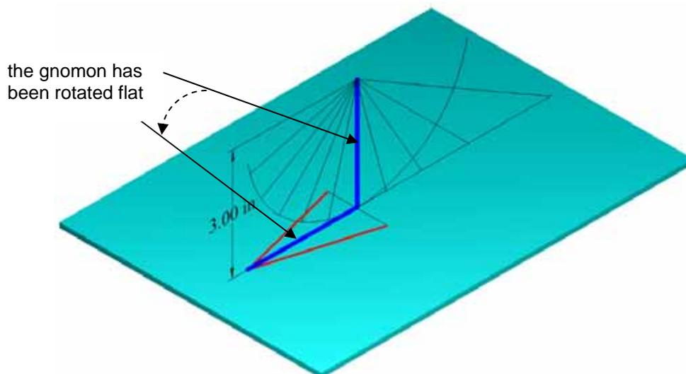
After the gnomon has been rotated flat, then the rays of light are projected from the nodus now on the dial plate.
