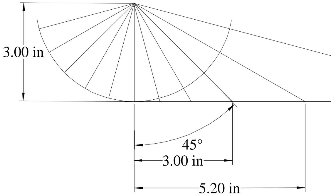
As an aside, the 60° radial shows a distance of 5.2 inches from the bottom of the circle with a radius of 3 inches. The distance along that horizontal line is the trigonometric tangent of the angle, times the radius.
